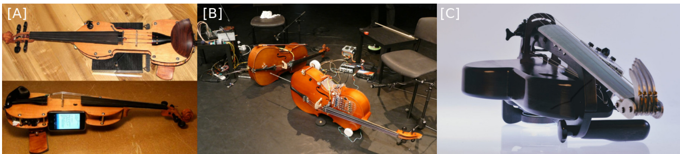
Figure 1: Case study instruments: [A] The Overtone Fiddle, [B] Feedback Cellos, [C] The Halldorphone
