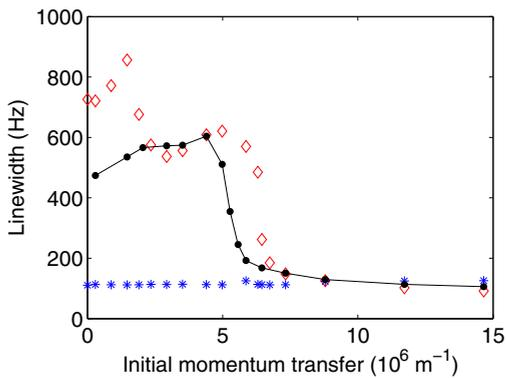
FIG. 3. (Color online) Linewidths of the condensate and the atom laser as a function of momentum kick for  $T = 384$  nK. Blue asterisks: condensate linewidth at outcoupling position. Red diamonds: atom laser beam linewidth. Black dots: Classical model of the linewidth of Newtonian particles exiting the system experiencing the fluctuating classical field of the trapped BEC as described in the text. All other parameters are the same as those in Fig. 1.
