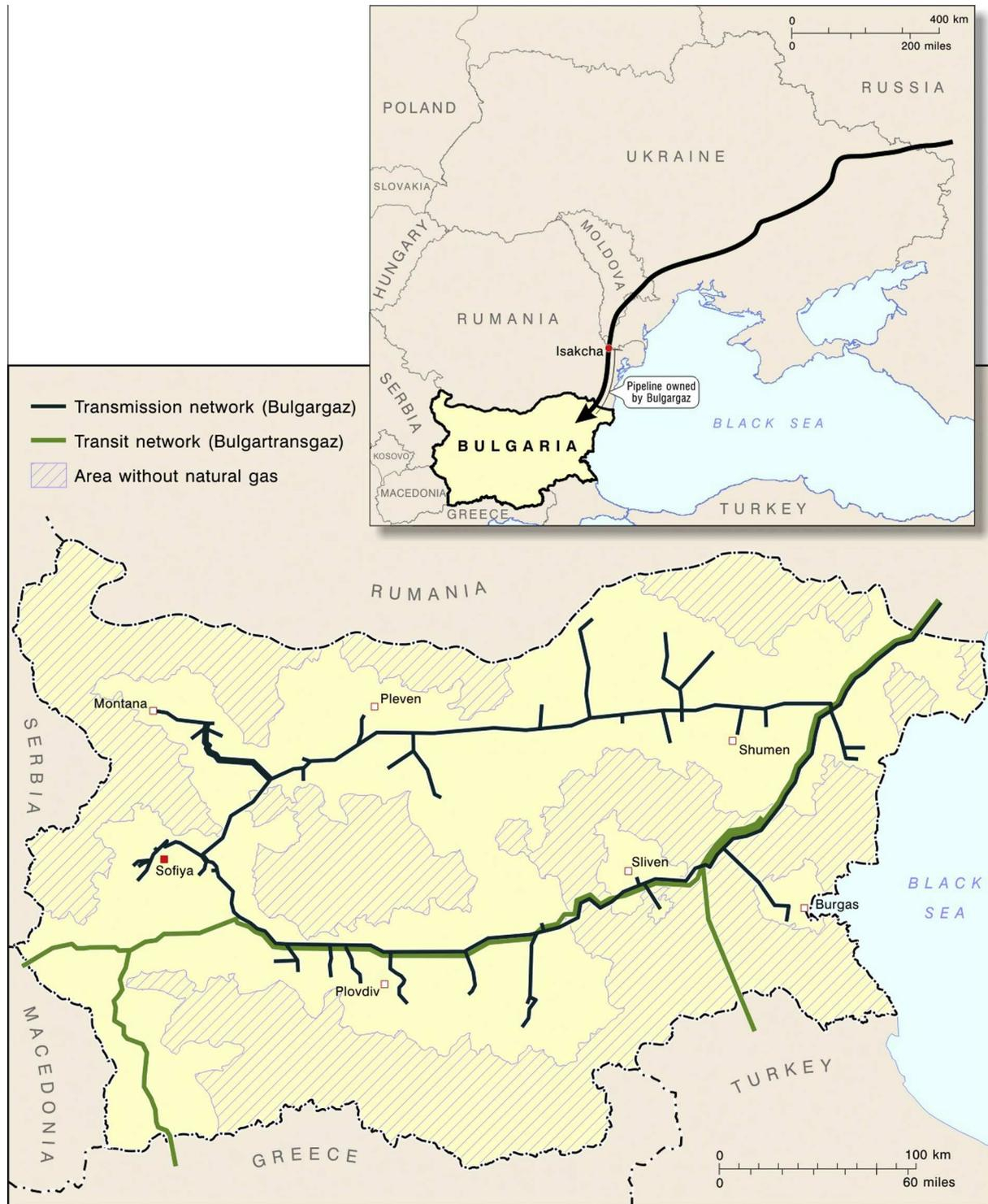
**Fig. 1.** Map of the Bulgarian natural gas pipeline network, which denotes areas with no access to natural gas.
