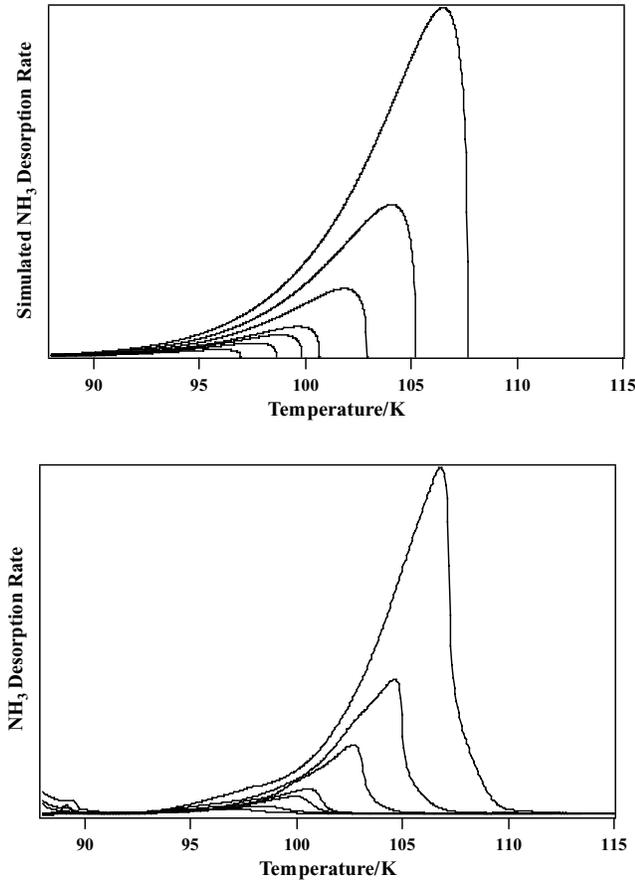
**Figure 2.** A comparison of experimental TPD spectra (bottom panel) and simulated TPD spectra (top panel) for  $\text{NH}_3$  adsorbed on HOPG at 88 K. The simulations were performed using the kinetic parameters given in Table 1.
