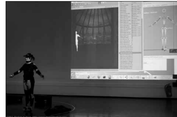
Figure 4. Realtime capture in a virtual environment using Animazoo/Sussex eMove tools.
