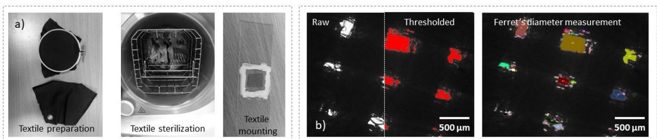
Fig 1. (a) Fabrics preparation for sterilization, b) Image analysis work flow for textiles pore measurement.
